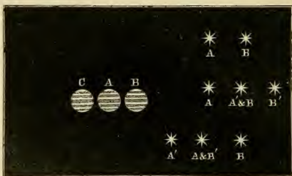
FIG. 105.—A B C, Images of Jupiter supposed to be touching; B being produced by duplication, C duplicate image on the other side of A. A B, Double Star; A, A' & B, B', the appearance when duplicate image is moved to the right; A', A & B', B, the same when moved to the left.
